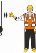
RAISE THE BOOM LOWER THE LOAD
