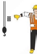
LOWER THE BOOM RAISE THE LOAD
