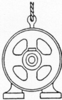
Vertical lift on eyebolt is good practice
