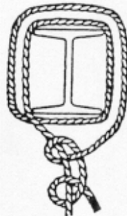
Bad Practice— Steel can cut rope
